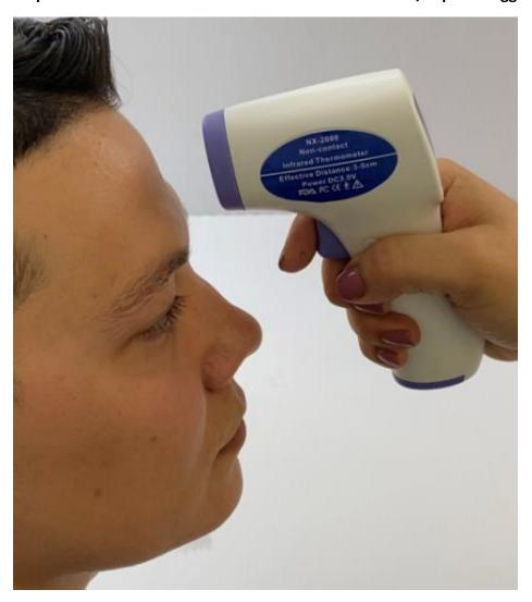
Step 7: Before moving onto the next person aim away from individual depress trigger and release/the screen will display "Lo" now you can take the next persons temperature
