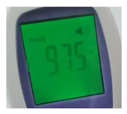
Step 6: Aim unit between 1 to 1 ½ inches from forehead/depress trigger until temp appears on screen
