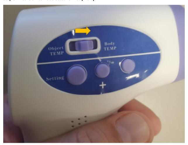
Step 4: Depress trigger for display to light up/ to change from Celsius to Fahrenheit press the setting button on the side of the unit once
